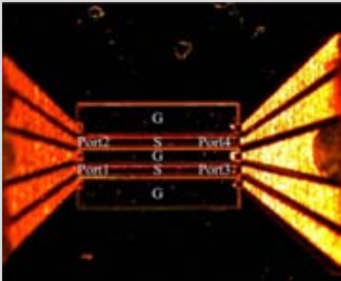
Shielding design of interconnects for 3D IC
