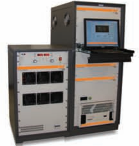
TGAR Automotive Transient Generator System, 60V/100 amps
